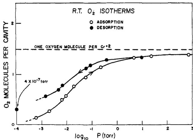
**Figure 1.** The oxygen chromium(II) exchanged anhydrous zeolite A room temperature isotherm. The adsorption is approximately 80% reversible at room temperature. The oxygen uptake also produces reversible color changes in the sample (see text).
